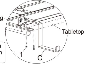
Fix the hook (C) on the side of supporting beam with screw (3) and use 5 x 5 allen key (2) to tighten. Then use hand drill to fix it on the tabletop.
