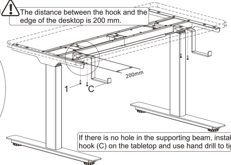
If there is no hole in the supporting beam, install the hook (C) on the tabletop and use hand drill to tighten.
