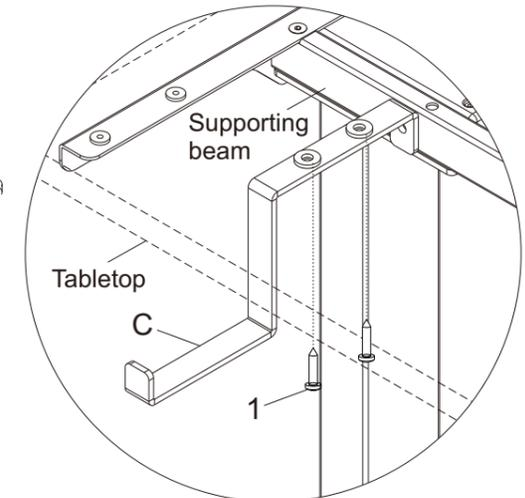
If there is no hole in the supporting beam, install the hook (C) on the tabletop and use hand drill to tighten.
