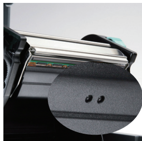
“Twin-Sensor” technology allows you to use a broad range of labels
