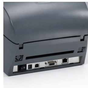
Available interface combinations include: - USB2.0, Serial and Ethernet - USB2.0 and Parallel
